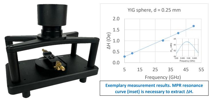
The hand-held tunable magnet allows performing the measurement in the **5** – **9 GHz** frequency range although it can be extended to the maximum range of 2 – 18 GHz by changing the spacer sleeves and the cavity support. The subwavelength cavity acts as a mechanical holder so it can be used up to the resonance frequency of its fundamental mode at ca. **60 GHz**. However, any use beyond 18 GHz requires the use of a stronger magnetic bias, e.g. with an external magnet.
