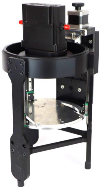
Fabry-Perot Open Resonator for Conductivity measurements
